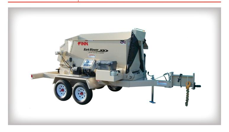
The FINN BB302 Bark Blower applies landscape mulch and other bulk materials with unprecedented efficiency, and eliminates the need for labor-intensive hand application. The 1.5 cubic yard hopper is perfect for smaller jobs and hard to reach areas.
